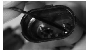
On the connector with the yellow wire, the pick should be inserted on the outside face of the terminal.
