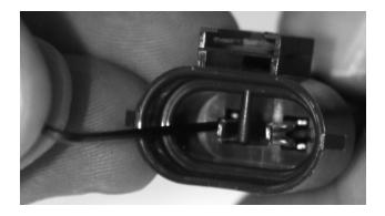
Reinsert the terminals as shown on the first page. The wire colors should now match the truck lighting harness (GM). If they do not, recheck the adapter.
