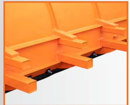
Reinforced Support 4" x 4" 3/16" lower posts and 3" x 4" x 3/16" upper posts with 72" wide x 4.5" tall post spacing
