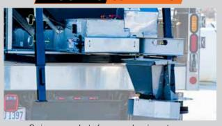
Swing away chute for easy cleaning, storage, and bulk unloading
