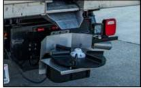
Removable spinner assembly for easy switch between spreader and dump applications
