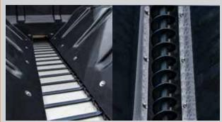
Full hopper length auger or chain feed for better material movement and less reliance on vibrator
