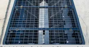
Patented double wall poly hopper built in our own factory and US 304 stainless steel trough
