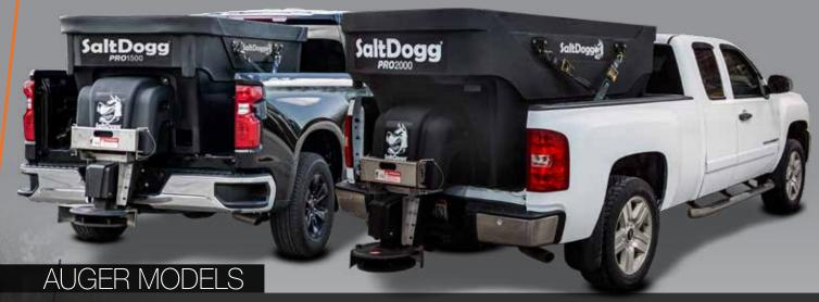
Feed Mechanism: 5-1/4 inch full length steel variable pitch auger, stainless steel trough Motor: Two 12V direct drive gear motors (3/4 HP for auger and 1/2 HP for spinner)
