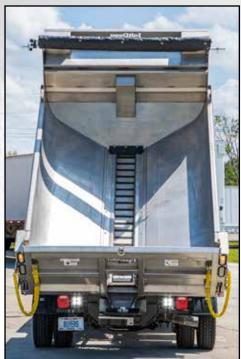
Cross member-free design makes the unit easy to clean with a low center of gravity that reduces strain powerful and reliable lifting and lowering on the vehicle
