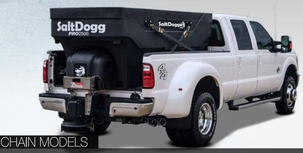
Feed Mechanism: 12 inch wide all steel pintle chain conveyor and stainless steel trough Motor: Two 121/ direct drive dear motors (3// HP for chain and 1/0 LID fo
