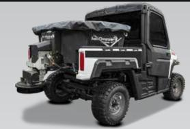
PRO8000 Electric Poly Spreaders 5-1/2 Inch Auger or 14-1/2 Inch Pintle Chain Feed 8 Cubic Yards pg. 16-17
