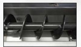
Heavy Duty 9 inch Dia. Auger for 92450SSA and 92452SSA 6 inch Dia. Auger for all other models
