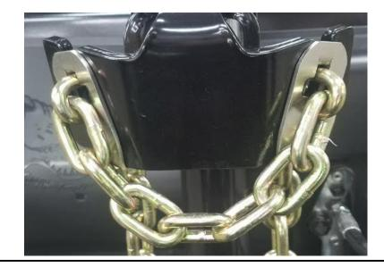
**CORRECTION** Install chains correctly and ensure that chain clip kit 16111410 is installed as shown.
