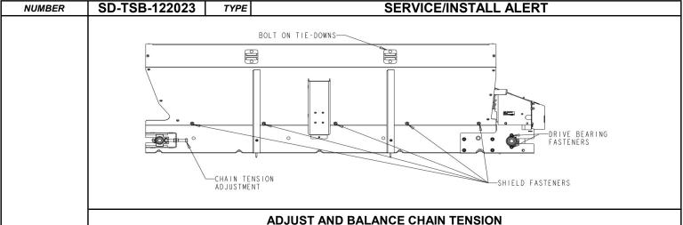
1. Adjust the chain tension using the idler adjust screws at the front the spreader using the standard instructions shown to the right. It is critical that the chain be tensioned evenly on BOTH sides. Excessive noise may be caused by an overly taught or unevenly tightened chain.
