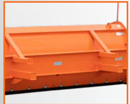
Reinforced Support 4" x 4" 3/16" lower posts and 3" x 4" x 3/16" upper posts with 68" wide x 4.5" tall post spacing
