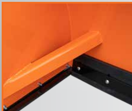
Rubber Edge 3/8" x 4" rubber edge mounting bracket, 1-1/2" x 10" premium rubber edge, 5/8-11, grade 5 carriage bolts
